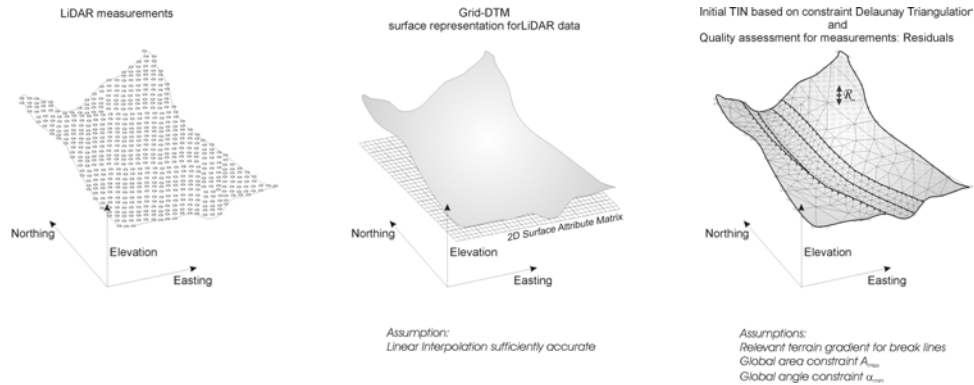
Figure 1. Gridding LiDAR data to derive break lines, being represented in a TIN.
