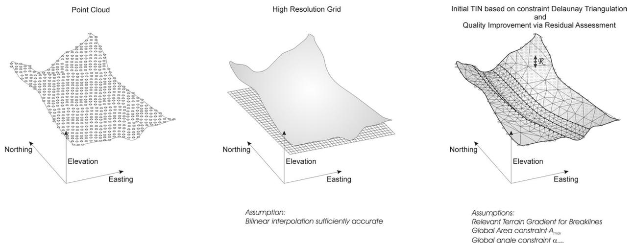
**Figure 2.** Modeling procedure - Meshing point clouds via automatic breakline detection based on slope classification on intermediate high resolution grids and subsequent representation in a TIN.
