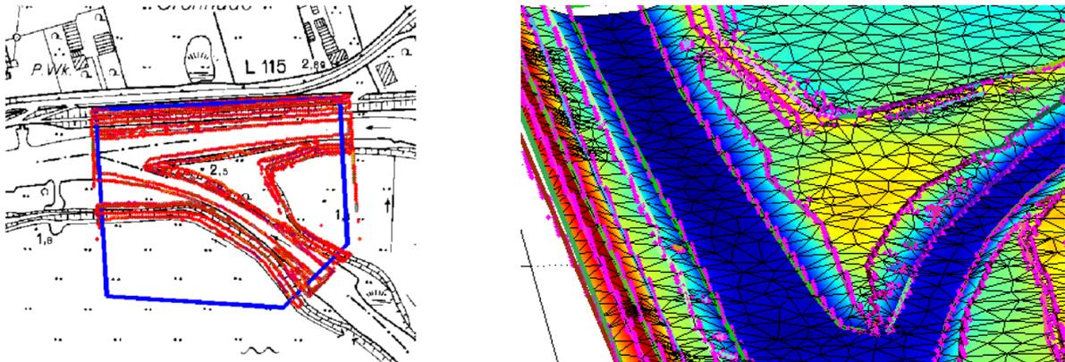
**Figure 2.** Model Application – River junction Stoer-Bramau, Northern Germany. Mesh (right) generated from breaklines delineated using a 10° threshold for One-Over Distance Slope computation on 1m HR grid.
