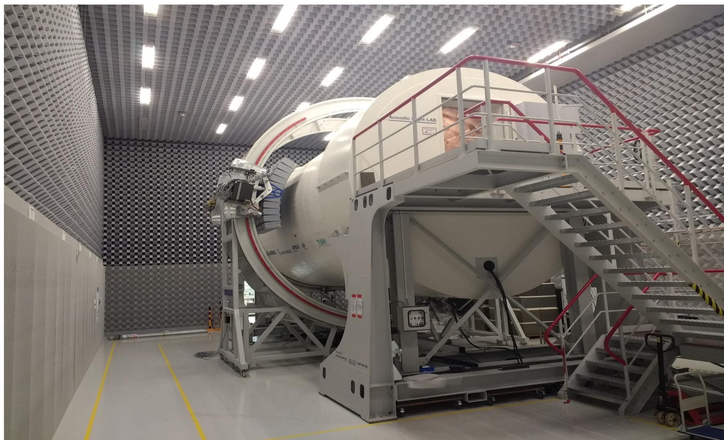
Figure 1: Loudspeaker array and fuselage set up. Source: Acoustic Flight LAB, ZAL Research Infrastructure
