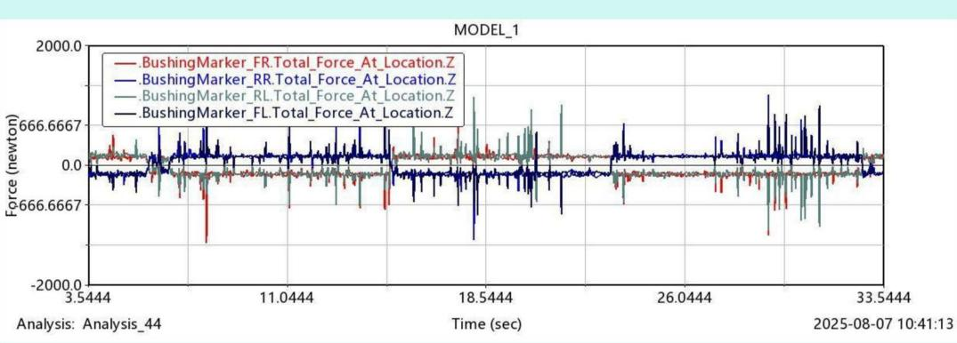
• Large, asymmetric spikes and drops, confirming uneven terrain loading and wheel unloading, which leads to reduced traction.
