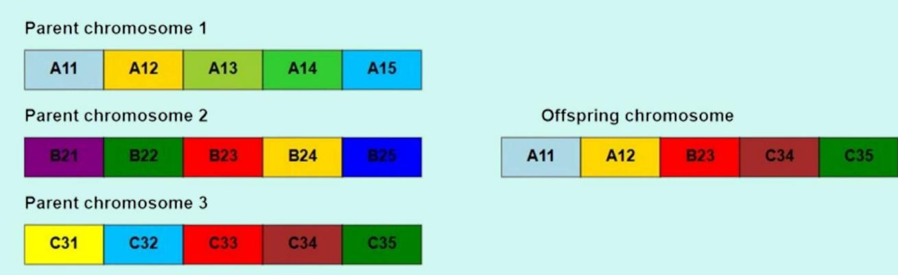
• Genetic algorithm crossover process for an AGV path. It combines segments from three different "parent" paths to create a new "offspring" path. This allows the algorithm to explore and create new, more efficient path combinations by mixing the best parts of existing solutions.
