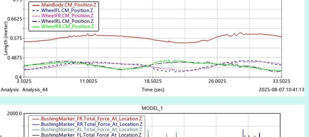
• The body line is much smoother than the wheel lines, demonstrating effective suspension isolation.
