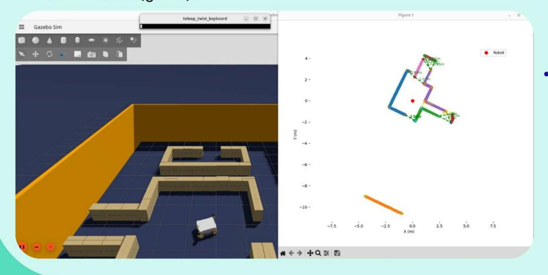
Robotics simulation for AMR navigation, visualizing real-time LiDAR data processing and pathway classification in an indoor testbed environment.
