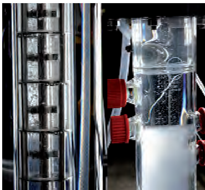
Lab scale counter current separation column for surfactant based separation processes
